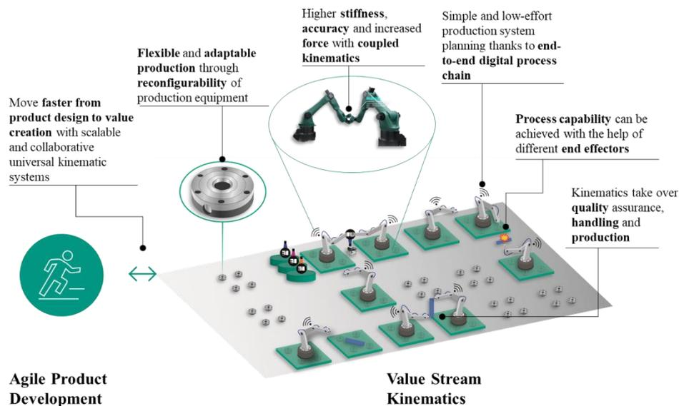
**Figure 1.1: Vision of the flexible production system 'Value Stream Kinematics' (Mühlbeier, Gönneheimer, Hausmann & Fleischer, 2020)**
