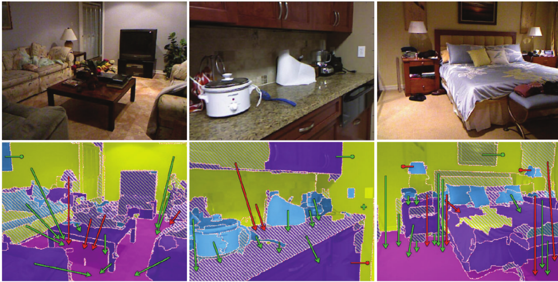
Figure 2.4.: Top row: Images of different indoor scenes. Bottom row: Segmentation results and inferred support relations (Correct relations are green arrows, wrong relations are red arrows). (taken from Silberman et al., 2012))
