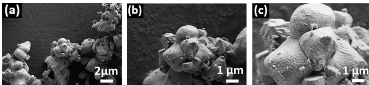
Figure 3.10. The SEM images of \text{CaS: Eu}^{2+} at a magnification of (a) 10,000x (b) 25,000x, and (c) 50,000x. The quasi-spheres have very high agglomeration that distorts their shapes. The particle size is >1 \mu\text{m} .
