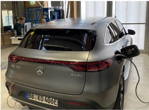
(a) EV (Mercedes-Benz EQC) connected to controllable charging station (KEBA [306])
