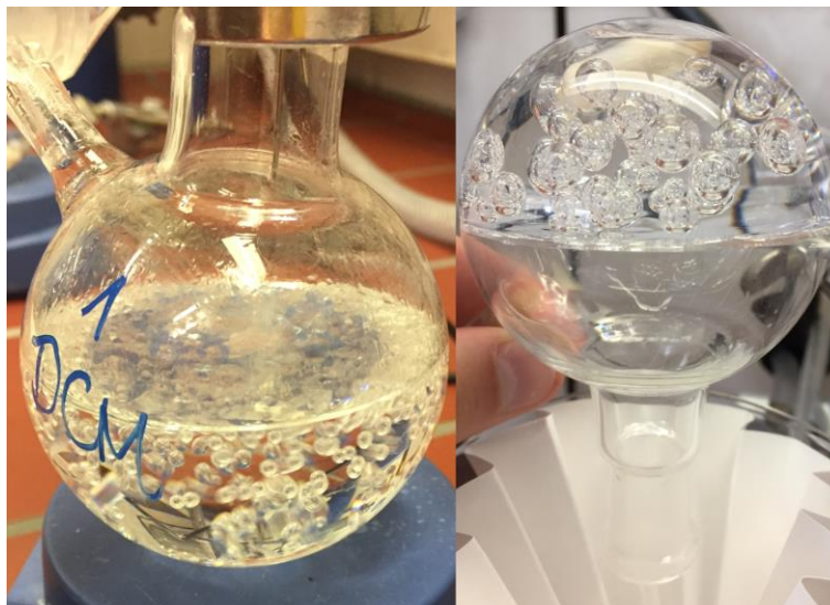
Figure 12 Pictures of the reduction of cellulose acetate with TMDS catalyzed by GaBr 3 in DCM.
