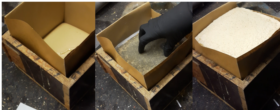
Figure 23 Foaming of polyol 2 with MDI. Left: 25 seconds after addition of MDI, center 30 seconds after addition of MDI, right: final foam 50 seconds after addition of MDI
