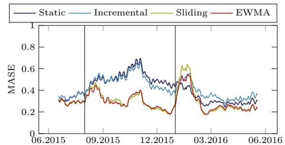
(a) The MASE of our method with different profiles on the concept drift Sudden 1.
