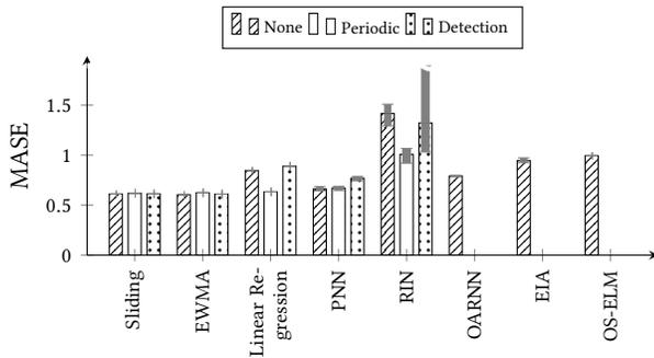
**Figure 6: The MASE of our method with the EWMA and Sliding profiles and the benchmarks on consumer U1 with the Sudden 1 concept drift at Position 1 for the three retraining strategies. The bars indicate the average MASE. The error bars show the worst and the best achieved MASE of the corresponding model.**
