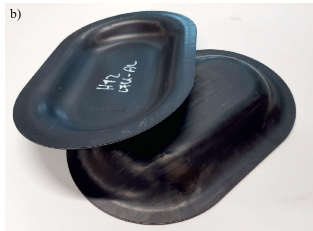
Fig. 2. Geometry of the 3D structures. (a) Target dimensions of the 3D structures with 0.5 mm thick elastomer layers; (b) Picture of hybrid (C-A-C and h-0.5 mm) 3D structures.
