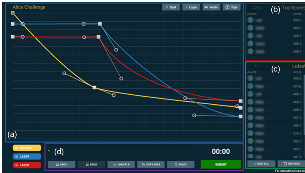
Fig. 15 The interface for the Alice Challenge, showing (a) the spline curves that the users could manipulate to control the time-dependent laser powers and magnetic field coil currents that controlled the final BEC atom number, (b) a top score list, (c) a list of the latest submissions and their scores, and (d) a control toolbar, including the estimated wait time. Players could take any other player’s solution [as shown in (b) and (c)] and modify it. Figure reproduced from Ref. 158.
