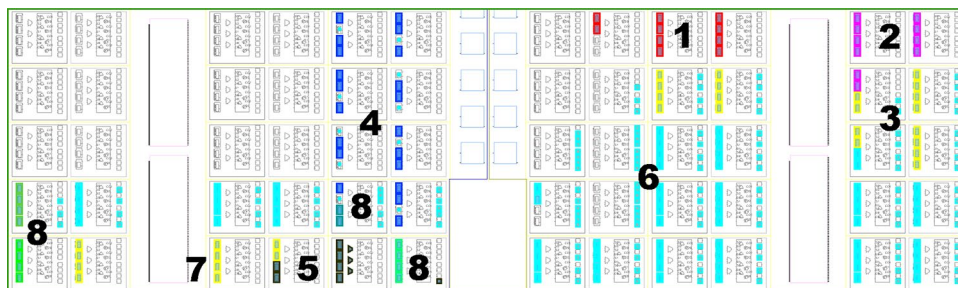
Figure 6 V-FPGA tile (type 9) placed using the manual placement strategy. Multiplexers of the PSM's top, right, bottom and left side are marked red (1), purple (2), yellow (3) and blue (4). The CLB is located at the bottom with the LUT, two internal multiplexers and D-flipflop colored in black (5). Sky blue color represents the config-
