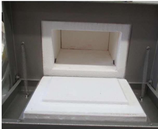
**Figure 4.21:** Interior of the high temperature oven used for the cladding corrosion experiment.
