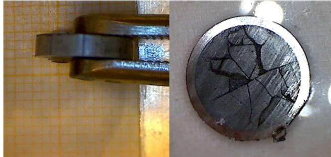
**Figure 4.7:** Pictures and dimension of the  $\text{UO}_x$  fuel segment used for inventory determination and spectroscopic analysis. The left picture shows the thickness of the cut fuel disk. The right picture shows the fractured surface of the irradiated fuel.
