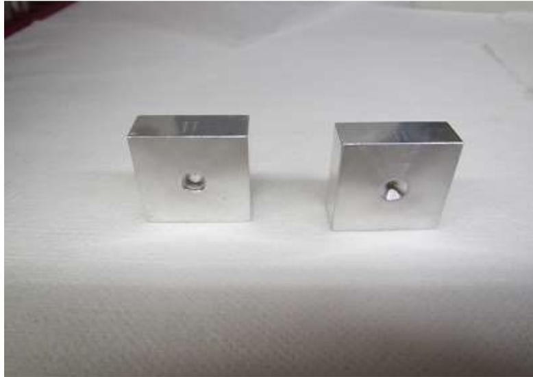
**Figure 4.16:** Sample holder designated for XAS measurements of SNF specimens.
