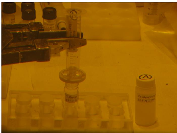
**Figure 4.14:** Precipitation of caesium and filtration with a 0.45 µm syringe filter.
