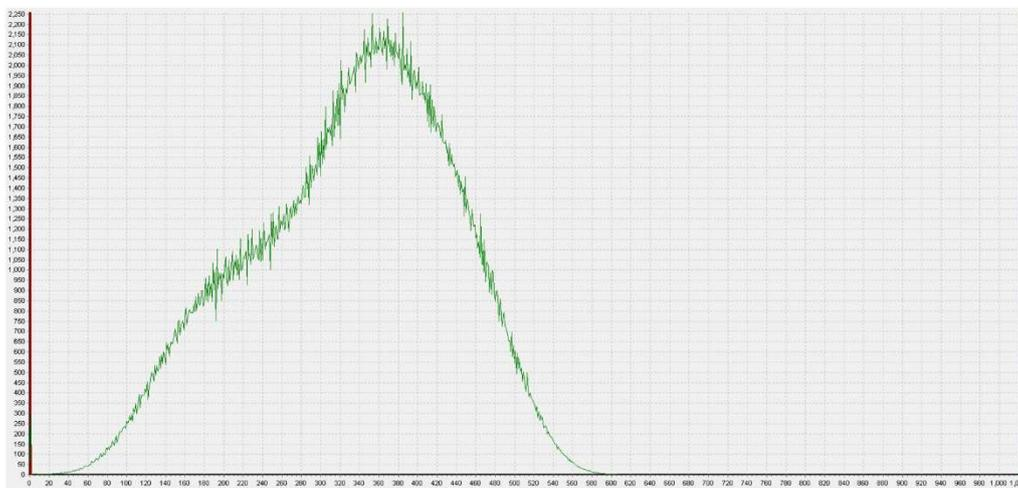
**Figure 4.2:** LSC spectrum of I-129 standard reference material displayed as frequency of impulses as a function of channel number.
