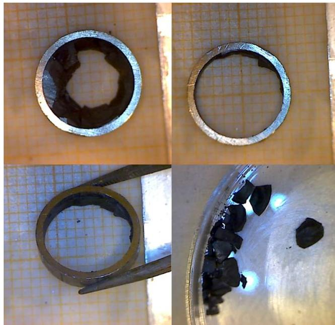
**Figure 4.8:** Defueling process of the high burn-up  $\text{UO}_x$  fuel. Upper left picture shows the segment with the central region already selectively defueled. Upper right and lower left picture feature the Zircaloy ring with fuel residue attached to it. Lower right picture shows the fragments obtained as a result of the defueling process.
