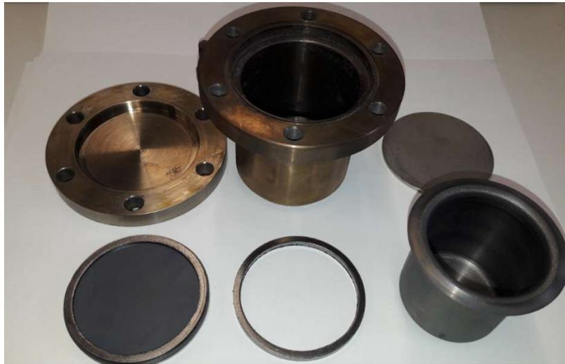
**Figure 4.19:** Autoclave, tantalum liner and graphite sealing rings for the cladding corrosion experiment.
