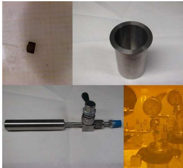
**Figure 4.10:** Fragment and material for gas phase analysis. Upper left picture features the  $\text{UO}_x$  fuel fragment used for fission gas analysis. Upper right picture shows the titanium liner later containing the specimen and solution. Lower left picture shows the SS-4CS-TW-50 gas sampling cylinder in detail and lower right picture depicts the reaction vessel equipped with a manometer and gas sampling connection.
