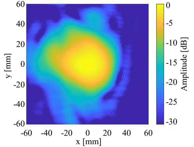
Fig. 6. Measured field intensity of the Gaussian beam after the quasi-optical output coupler at 170 GHz. The measurement is performed at the position of the gyrotron output window. The pixel size is 1x1 mm. The field intensity is normalized to its maximum.
