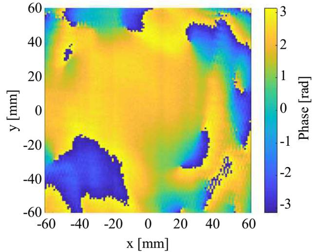
Fig. 7. Measured phase of the Gaussian beam after the quasi-optical output coupler at 170 GHz. The measurement is performed at the position of the gyrotron output window. The pixel size is 1x1 mm.
