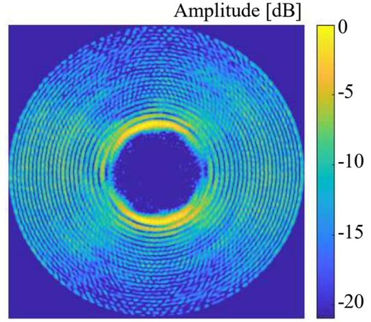
Fig. 3. Measured E-field intensity pattern of the  $TE_{40,23}$  mode operating at 204.071 GHz with a pixel size of 0.25x0.25 mm. In this figure the y-polarization is presented.
