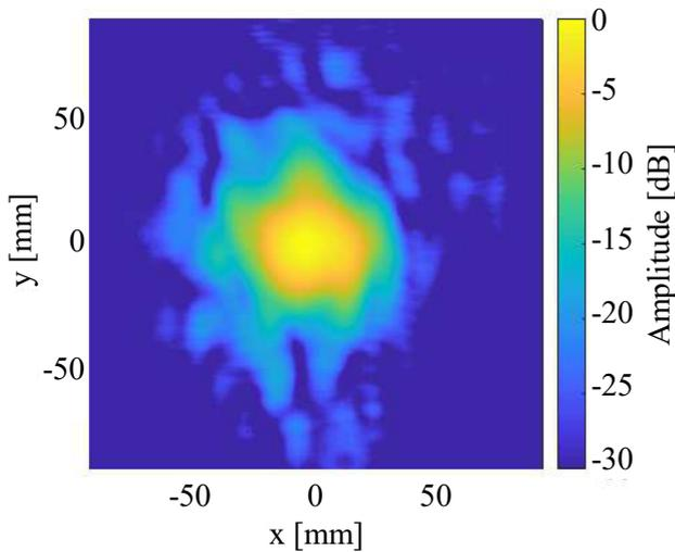
Fig. 9. Measured field intensity of the Gaussian beam after the quasi-optical output coupler at 204 GHz. The measurement is performed at the position of the gyrotron output window. The pixel size is 0.5x0.5 mm. The field intensity is normalized to its maximum.
