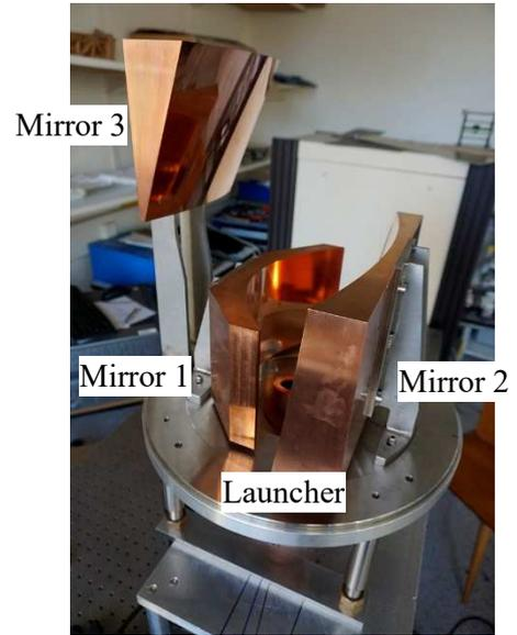
Fig. 4. Photo of the measurement setup for the evaluation of the quasi-optical gyrotron output system consisting of a launcher and three mirrors at 170 GHz and 204 GHz. The quasi-optical output coupler is assembled onto the mode generator setup.
