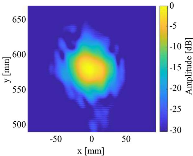
Fig. 8. Simulation of the field intensity of the Gaussian beam after the quasi-optical output coupler at 204 GHz. The field intensity is normalized to its maximum.
