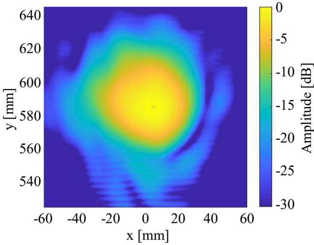
Fig. 5. Simulation of the field intensity of the Gaussian beam after the quasi-optical output coupler at 170 GHz. The field intensity is normalized to its maximum.
