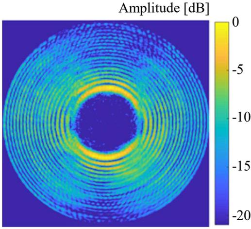
Fig. 2. Measured E-field intensity pattern of the  $TE_{34,19}$  mode operating at 170.325 GHz with a pixel size of 0.25x0.25 mm. In this figure the y-polarization is presented.
