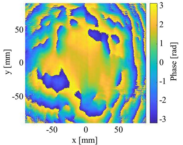
Fig. 10. Measured phase of the Gaussian beam after the quasi-optical output coupler at 204 GHz. The measurement is performed at the position of the gyrotron output window. The pixel size is 0.5x0.5 mm.
