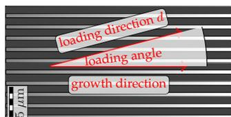
(b) Sketch of a longitudinal section indicating the loading angle
