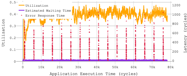
Figure A.18: Packet waiting time and error response time over the execution time of MM (-o3), f = 1 .
