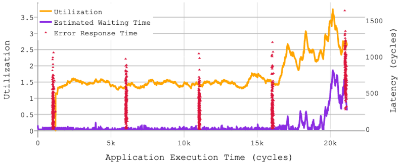
Figure A.8: Packet waiting time and error response time over the execution time of Quicksort (-o3) , f = 3 .
