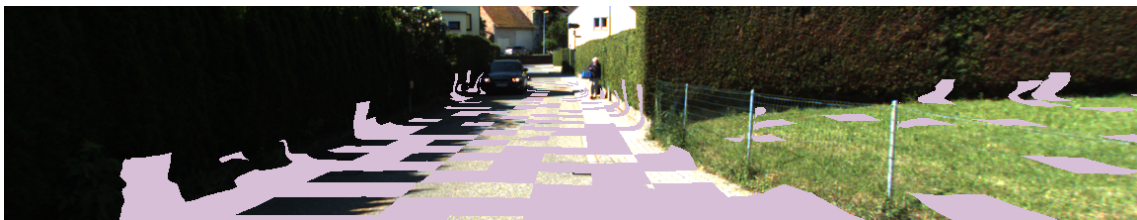
Figure 3.6: Visualization of the areas that GndNet segmented as the ground on the pseudo-lidar point cloud. Segmented ground is colored as purple. Considered is KITTI-360 [82] sequence 0005 and time point 752.
