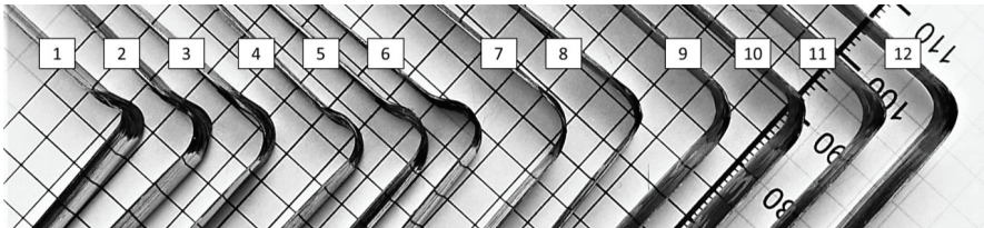
Figure 5-16: Variation of the bend shape depending on t_0 and b_0 . (Image source: (A_Bachtin 2020))
