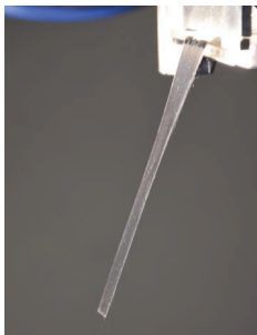
Figure 3-7: Bending of a heated area by gravitational forces
