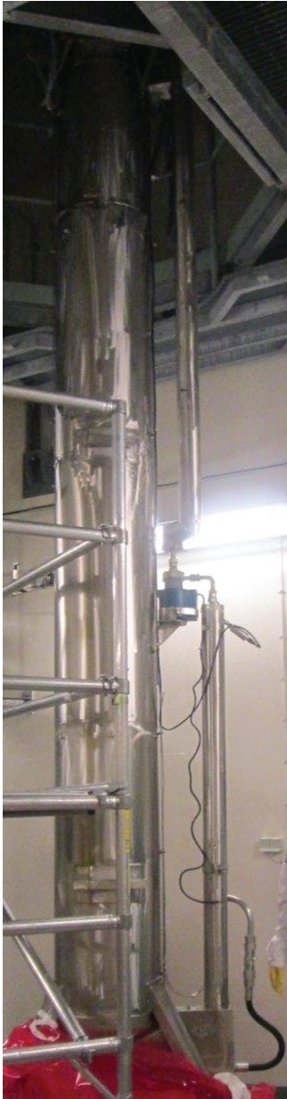
Fig. 1. Photo of the calorimeter used for measurements of decay heat at the Clab.
