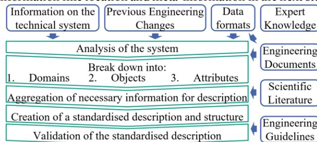
Fig. 4. Introduced approach to create a standardised description
