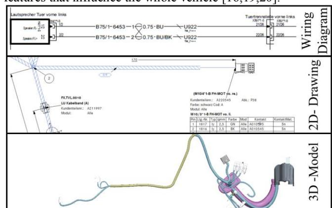
Fig. 1. Domains in the wiring harness development process
