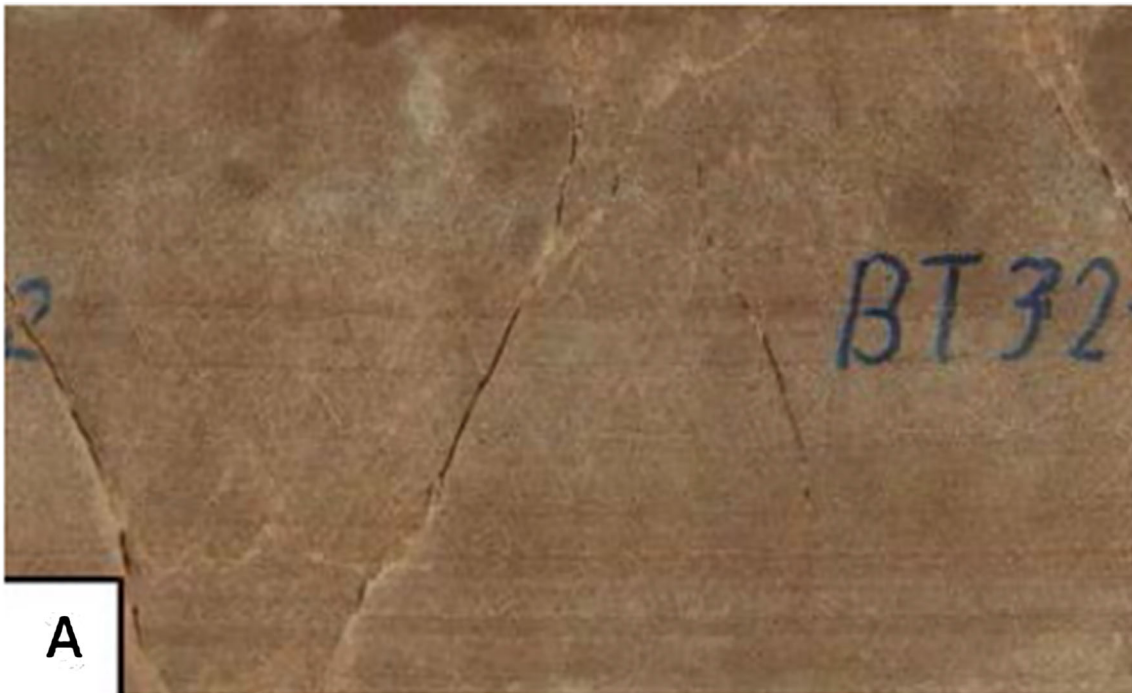
Fig. 11 Unrolled combined photographs of a sandstone sample after a multi-stage triaxial test with \sigma'_3 > c' [18]
