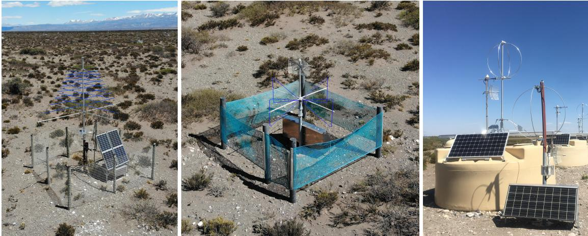
**Figure 3.4.:** Pictures of 3 AERA antenna stations, each with a different radio antenna (from left or right): LPDA, Butterfly, (AERA-)SALLA. For LPDA and Butterfly the sensitive antenna elements are highlighted in blue.
