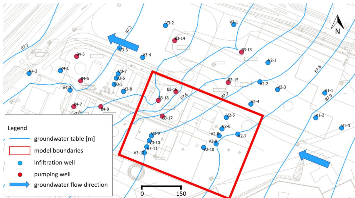
Figure 18. The groundwater water flow path. The boundaries of the reactive transport model (blue isolines are result from ARCADIS (2012)).
