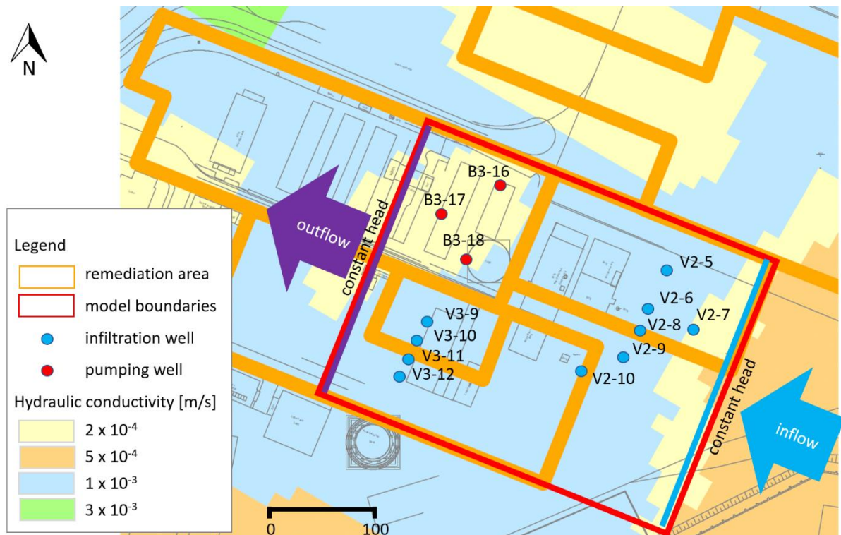
Figure 20. Boundary conditions. Hydraulic conductivity distribution in the first layer (the distribution based on the data from ARCADIS (2012)).
