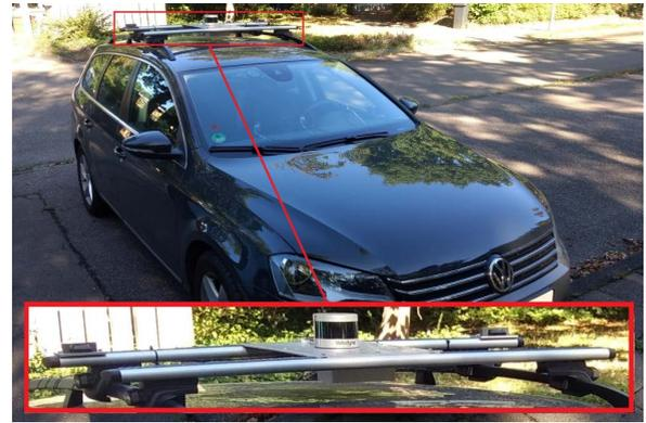
FIGURE 1. Test vehicle with sensor setup on the roof.
