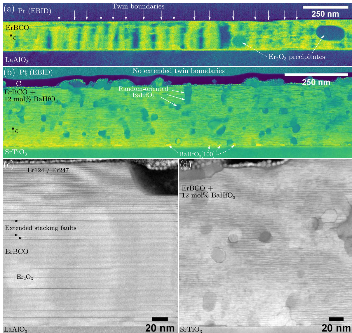
Figure 5.34: Comparison of pristine (a,c) ErBCO and (b,d) ErBCO-BaHfO 3 films. (a and b) Representative color-coded LAADF-STEM cross-section image of (a) a pristine ErBCO and (b) an ErBCO-BHO films. The presence of nanoparticles (Er 2 O 3 and BHO) disrupts the ordered twin-boundary arrangement. (c and d) HAADF-STEM image of the microstructure revealing a significantly higher stacking-fault density for the ErBCO-BHO film. (d) Some of the short stacking faults may result from TEM-sample degradation in air. (c) A high density of extended stacking faults (marked with arrows) close to the pristine ErBCO film's surface leads to the formation of Er124 and Er247.
