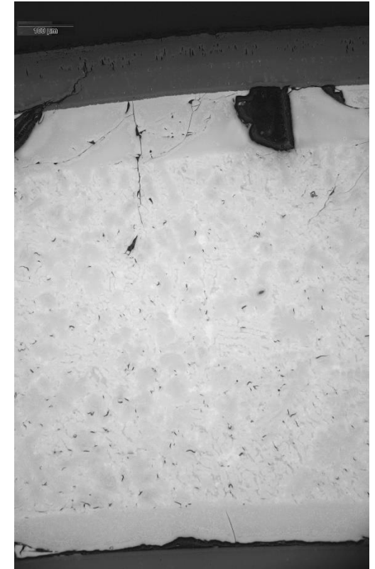
315°: absence of inner oxide layer
