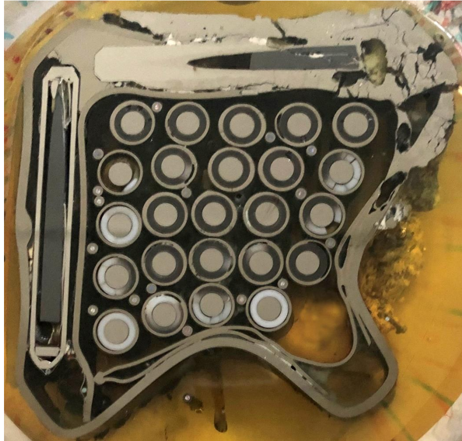
Figure 190 QUENCH-20; Bundle cross section at the elevation of 450 mm; influence of higher temperatures in the bundle (melt relocation from above and melting of cladding inner \beta -Zr layer) and at the shroud position of 0^\circ (eutectic interaction B_4C pin with stainless steel blade). Not changed white pellets inside rods without melt.
