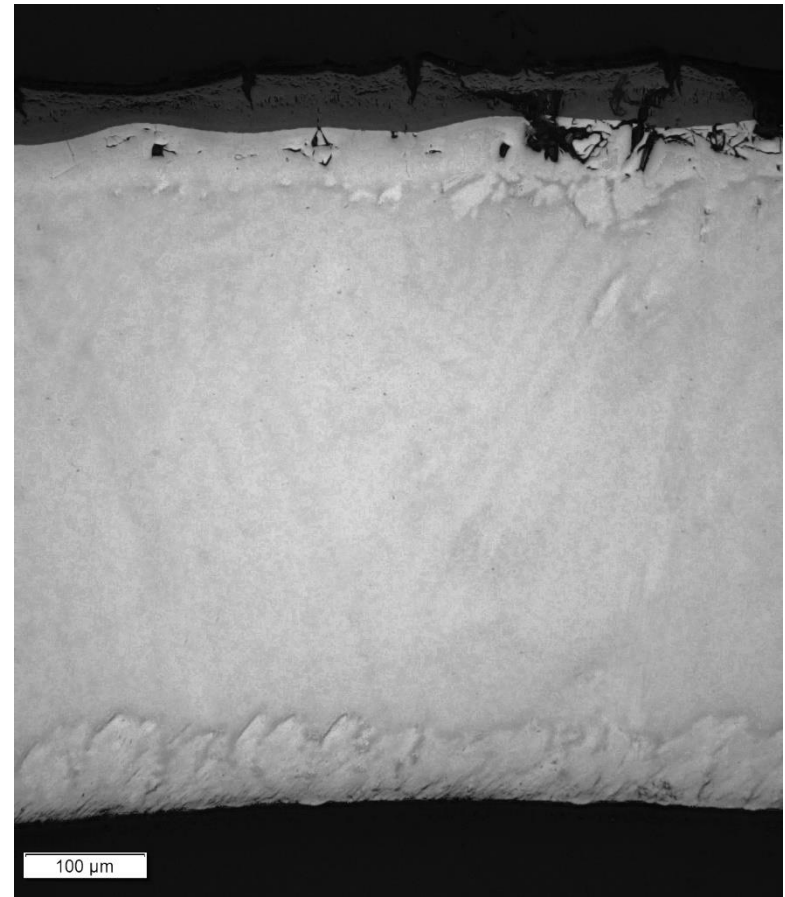
Figure 189 QUENCH-20; rod #24 at elevation 555 mm: cladding structure with melt formed at inner cladding surface.
