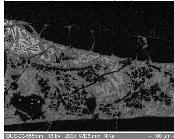
penetration of Ni (from spacer grid) into cladding melt
