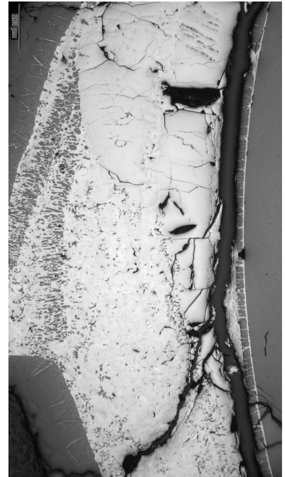
180°: cladding metal relocated from above
