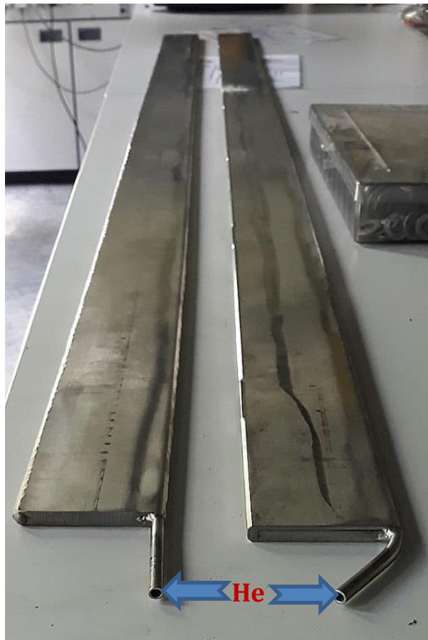
absorber blades filled with B 4 C pins and prepared for filling with He
