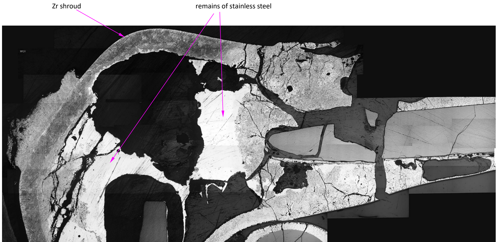
Figure 132 QUENCH-20; interaction of stainless steel blade with ZIRLO channel box and shroud at elevation 650 mm and bundle azimuth 0° (left side of B 4 C pin).
