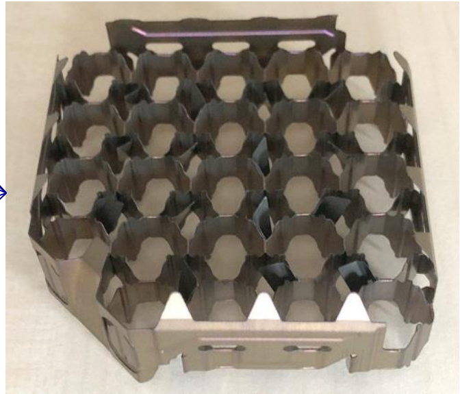
sleeve type spacer grid Inconel X750
