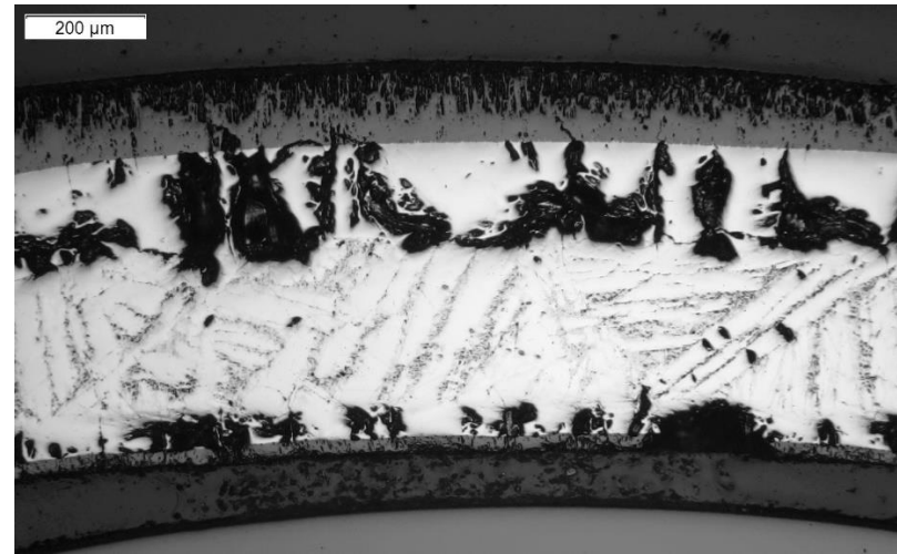
90°: thick prior \beta -Zr layer
