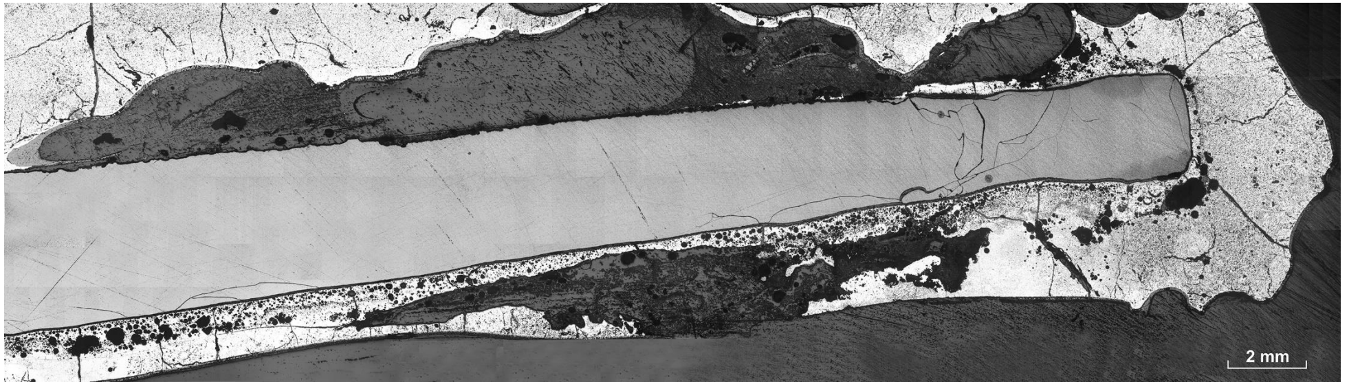
Figure 130 QUENCH-20; interaction of B 4 C pin with stainless steel blade and channel box at elevation 650 mm and bundle azimuth 0° (right side of B 4 C pin).
