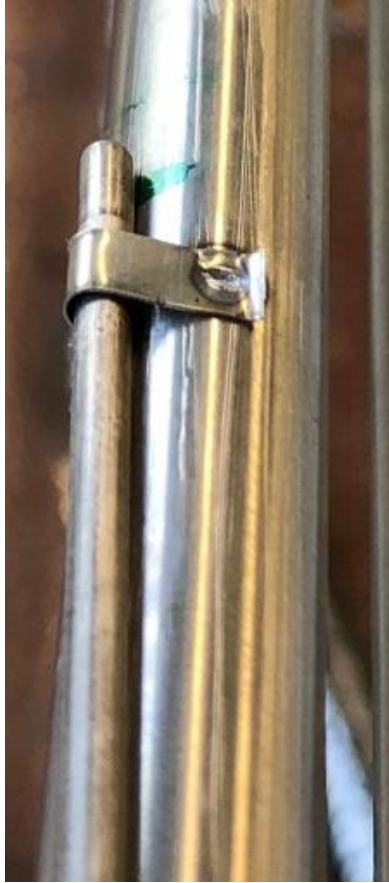
high temperature TC at cladding surface
