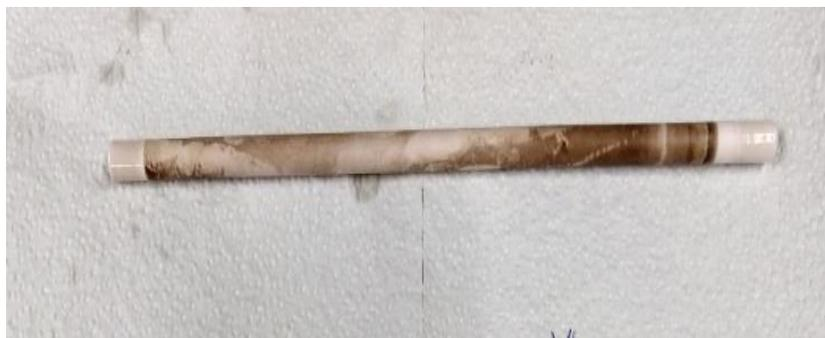
**Figure SB3** Fouling on the permeate side of the membrane after backwash cycles (experiment 3.4).
