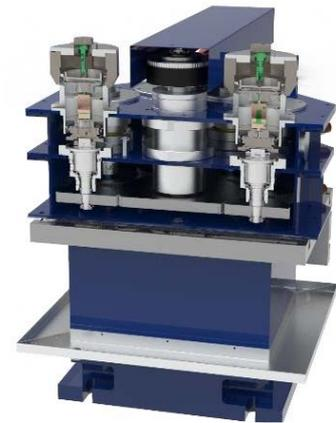
Figure 6. Validation environment for testing graphite lubricated axial ball bearings
