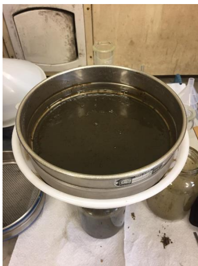
Figure SB1. Raw pig manure sieving through 1mm sieve
