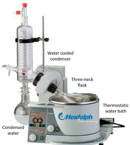
Figure SB2. Lab scale vacuum evaporation system.
