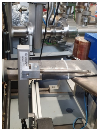
Figure 2: A scintillator detector (without the lead shield) being calibrated with ^{137}\text{Ce} radioactive source at the KARA storage ring
