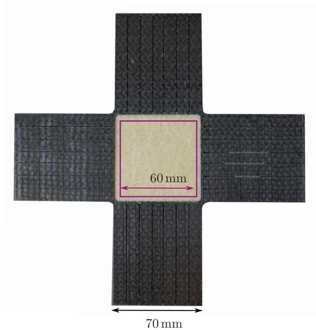
Figure 4.8: Biaxial specimen; use in: biaxial testing device, for details see Section 4.5.1.
