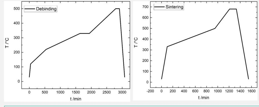
The soluble pre-debindered samples were then thermally debindered at 500 °C and subsequently sintered at 680 °C. Sintering was carried out under air conditions and under vacuum.
