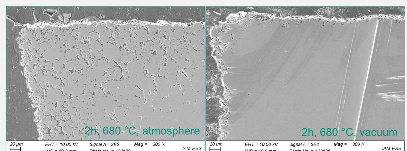
Compared to vacuum sintering, small bubbles can still be found in the component during sintering under air conditions, and the surface layer with an open porosity is somewhat thicker.
