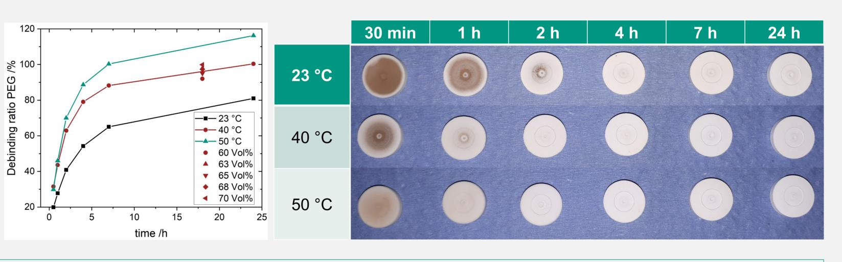
Dependence of the debinding rate of PEG on time and water temperature. After 16 h, a 90% debinding rate is achieved at a water temperature of 40°C, which is sufficient for the further process.
