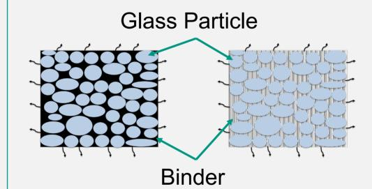
Schematic process of soluble pre-debinding: (left) in the green state, (right) after soluble pre-debinding
