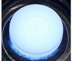
After sintering, glass samples are translucent because of the thin open
