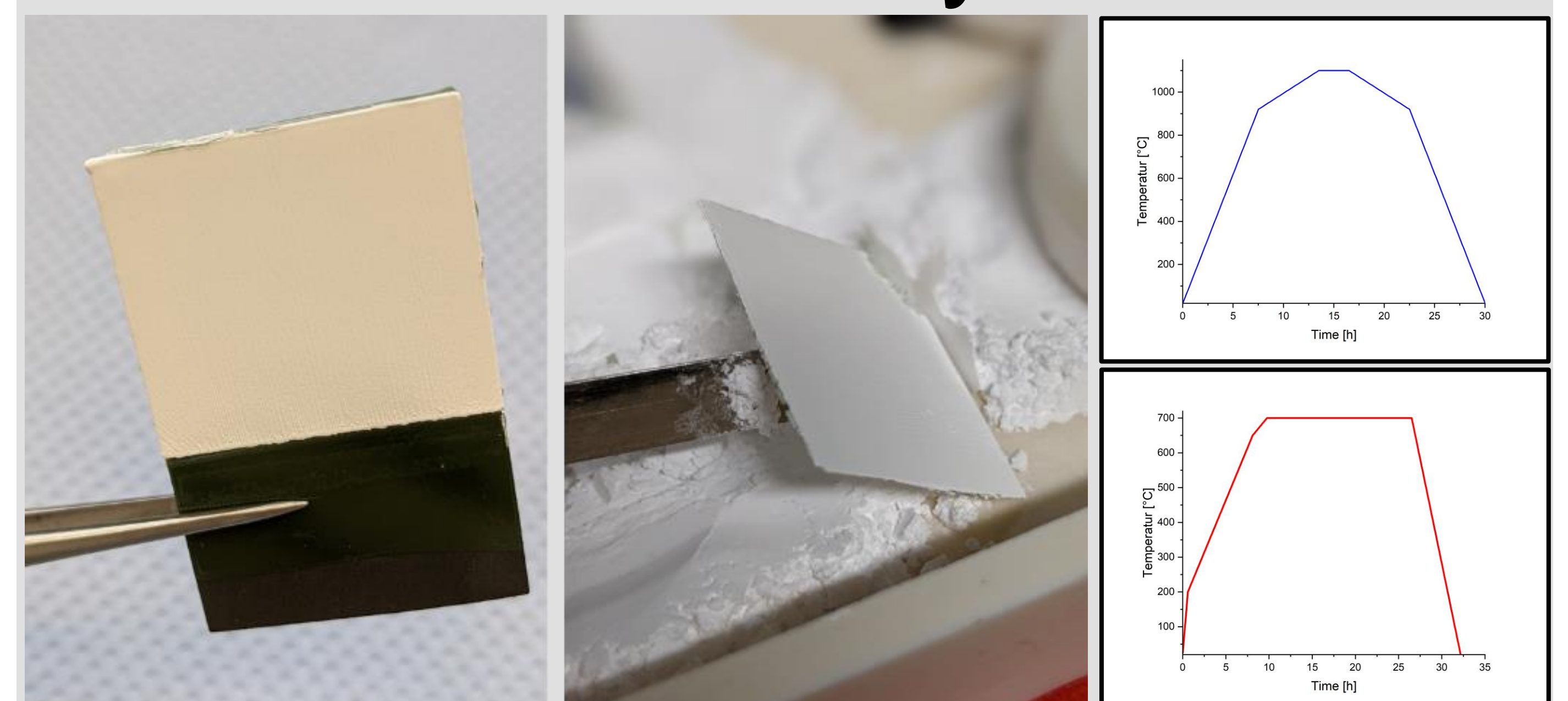
Fig. 7: from left to right: Ceramic composite layer on graphite substrate, layer after debinding and sintering, debinding (red) and sintering (blue) temperature programm
