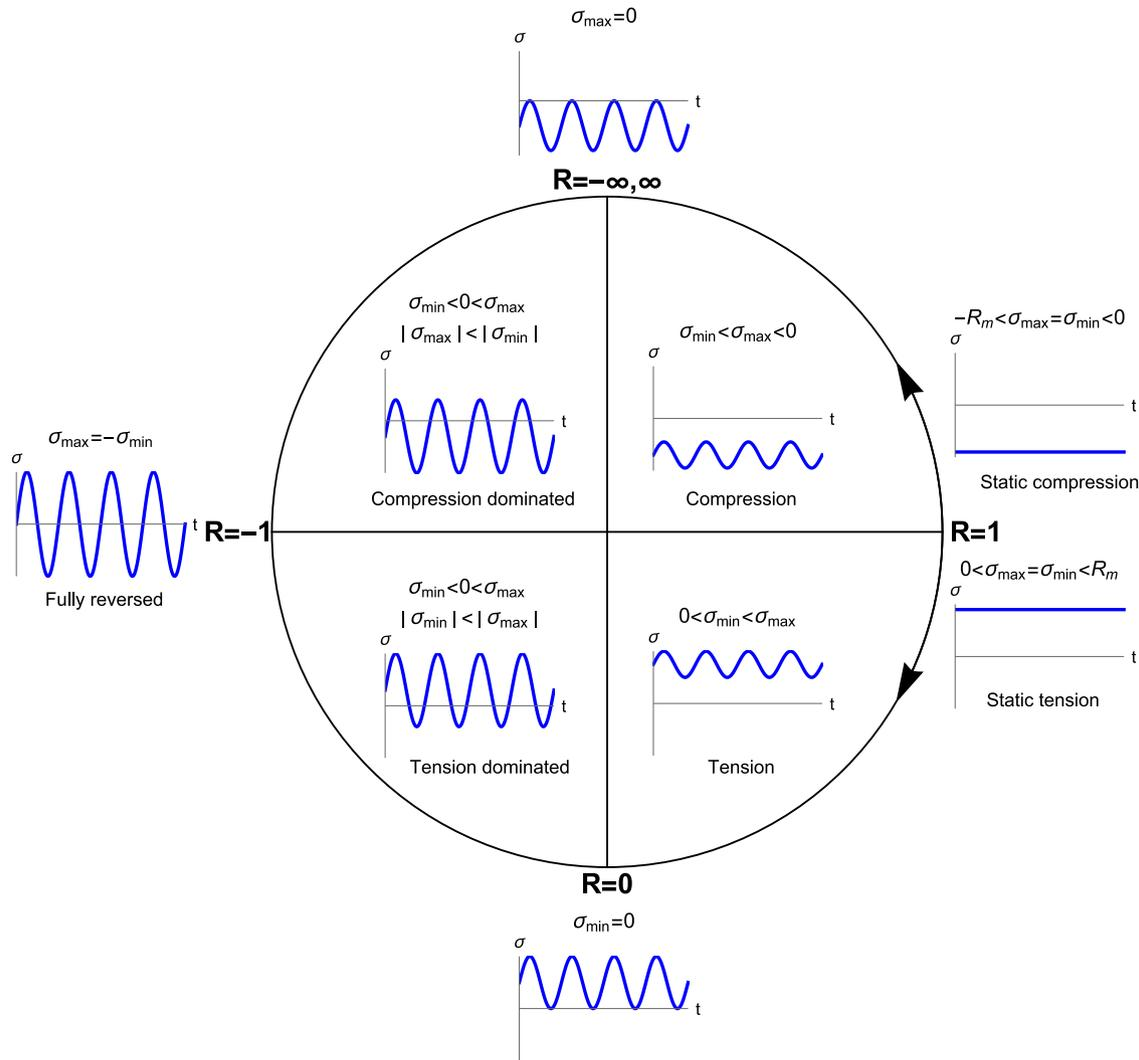
Fig. 1. Effects of the stress ratio on the loading wave geometry.  $|\sigma_{max}| < R_m$ ,  $|\sigma_{min}| < R_m$ .
