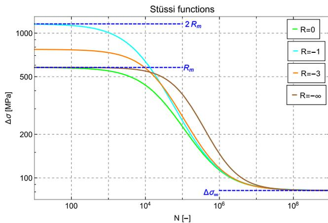
Fig. 4.  $S-N$  or Wöhler curves based on the Stüssi function for different stress ratios.
