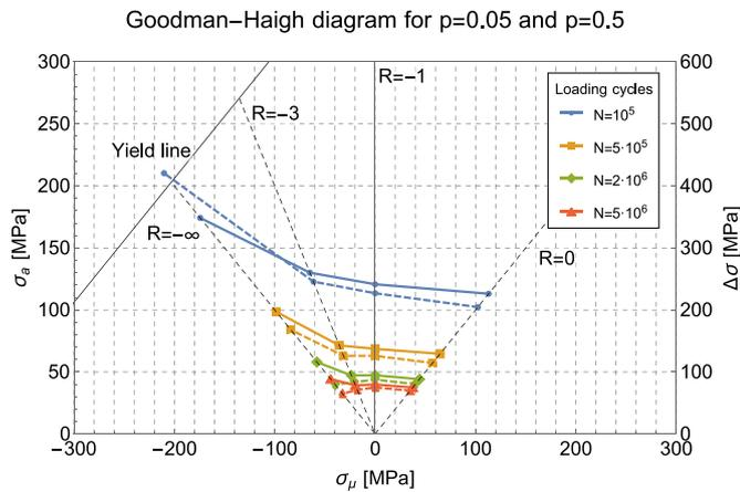
Fig. 10. Goodman-Haigh diagram for probabilities  $p = 0.05$  and  $p = 0.5$ .
