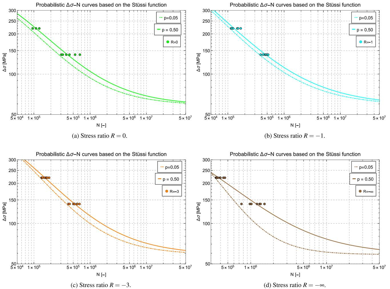
Fig. 9. Probabilistic S-N curves for different stress ratios  $R = 0, -1, -3, -\infty$  and for a probability  $p = 0.5, 0.05$ .
