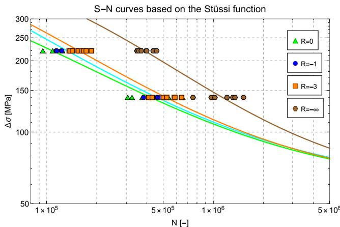
Fig. 7.  $S-N$  curves for different stress ratios.
