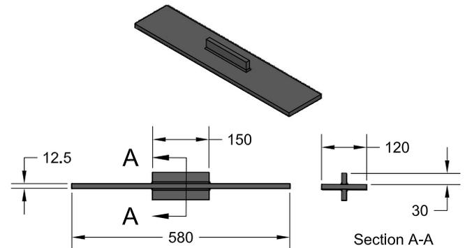
Fig. 5. Geometry of the specimen.
