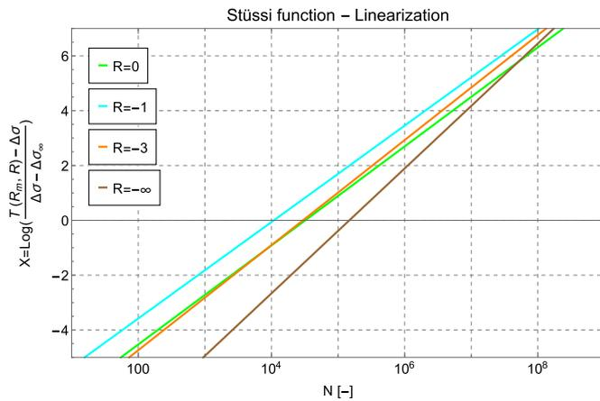
Fig. 3. Linear regressions of the Stüssi function  $S(N, R)$  for different stress ratios.
