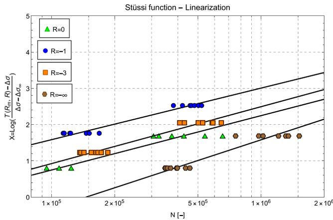
Fig. 6. Linear regression of the Stüssi function  $S(N, R)$ .
