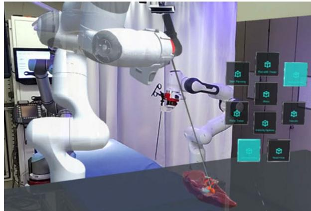
**Fig. 1:** Virtual scene with robot and menu in the foreground, and real operating room table and robot in the background.
