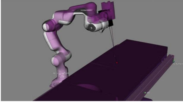
**Fig. 2:** Visualization of the planned trajectory. Old robot state in original colors, new state in magenta.
