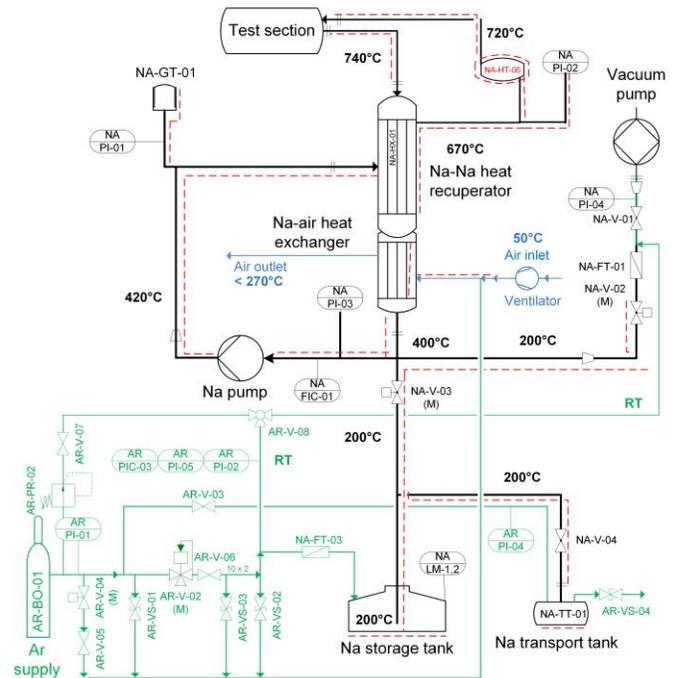
**Figure 2** Piping and instrumentation diagram of the SOLTEC-1, -2 facilities
