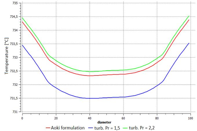
**Figure 9** Sodium temperature distribution through the model for a sodium flow rate of 137 kg/h at the maximal specified temperature of 720°C
