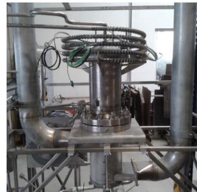
**Figure 3** Combined sodium-sodium heat recuperator / sodium-air heat exchanger, the high temperature heater and the air cooling system
