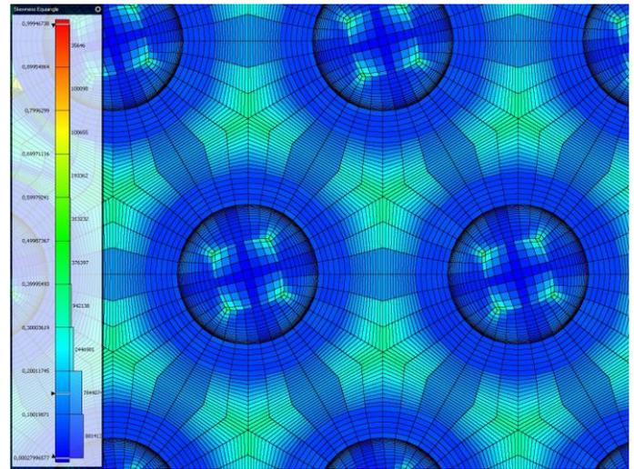
**Figure 5** Mesh skewness in cross-section through the sodium-sodium heat recuperator
