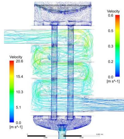
**Figure 7** Sodium velocity vectors and air streamlines in the sodium-air heat exchanger
