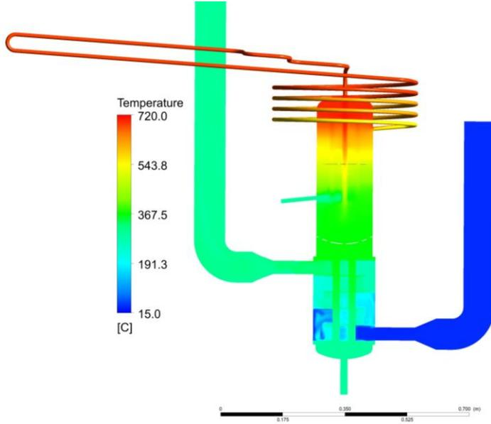
**Figure 8** Sodium and air temperature distribution through the model for a sodium flow rate of 125 kg/h at the maximal specified temperature of 720°C
