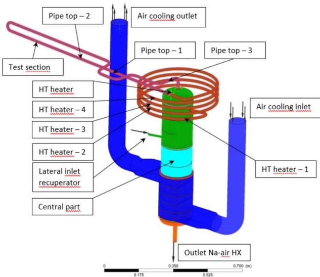
**Figure 4** View of the CFD model exhibiting inlet and outlet conditions and positions of thermocouples
