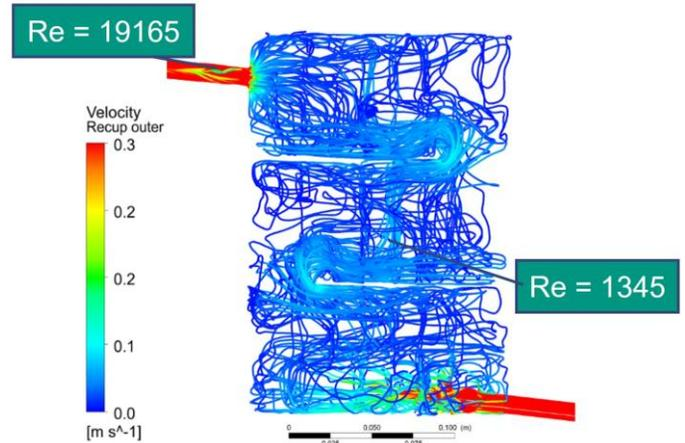
**Figure 6** Velocity streamlines in the Na-Na heat recuperator for the case with  $\dot{m} = 137$  kg/h
