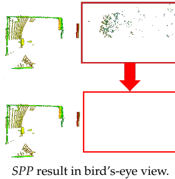
Figure 4.3 Outlier filtering with SPP conducted with a min. of 10 neighbors in r = 0.15 m and points inside the red box were removed as outliers.
