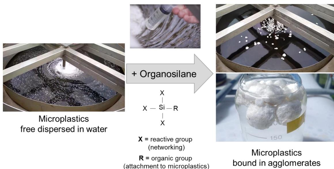
**Figure 1-11:** Scheme showing removal of microplastics using organosilanes. 50 mg / l PE and PP (50:50) are removed from 2 m<sup>3</sup> drinking water in a model experiment [82].
