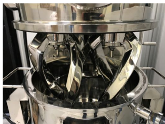
Figure 2.2: Mixing tool of the kneader Inoue Trimix TX-15 (MVT-VM, KIT).
