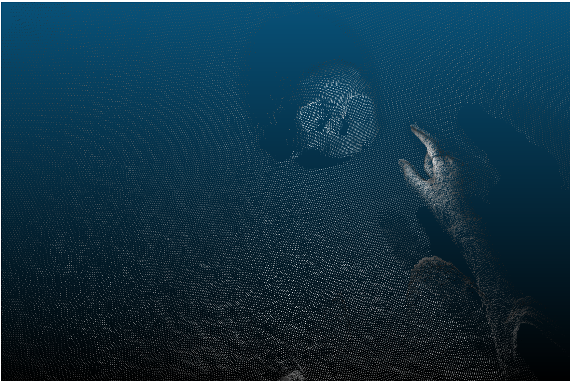
Figure 5.36.: Recorded point cloud of the short throw depth stream.
