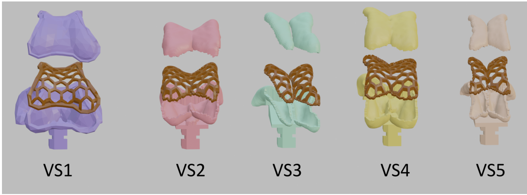
Figure 5.4.: Molds to model the ventricular systems from modeling clay.
