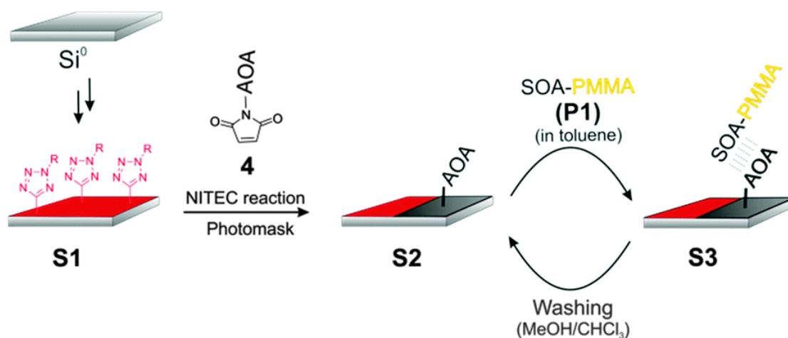
**Figure 1.6** Schematic representation of the synthetic route to the patterned immobilization of symmetrical oligoamide-asymmetric-polymethylmethacrylate (SOA-PMMA) on a silicon wafer. The wafer was globally functionalized with tetrazoles (S1) and partly functionalized with AOA-Mal (4) via a photo-induced NITEC reaction employing a shadow mask resulting in S2. SOA-PMMA (P1) was repeatedly immobilized and washed off the AOA-functionalized part of S2/S3. Adapted from Ref.<sup>96</sup>
