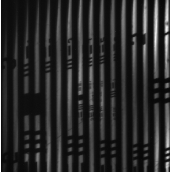
Figure 5: Signal on the image sensor during narrow-banded illumination of a USAF target. The USAF target was illuminated in transmission with a central wavelength of 632 nm. The half-width of the illumination spectrum was 10 nm.
