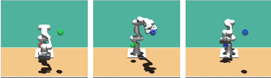
Figure 8: Virtual part of the setup for collecting human demonstrations for the Panda Reacher task. Starting from a resting position (left), the human demonstrator is tasked to reach the intermediate target (green). Once reached, both targets change color (middle). The task is successful if both targets have been reached (right).
