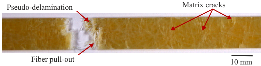
Figure 5.10: DiCo SMC specimen that was tested at a maximum stress of 120 MPa and failed after approximately 3 \cdot 10^5 cycles due to fatigue.
