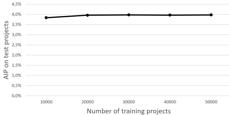
Figure 5.30: AIP performance indicator for the tuned NN-CONVID-FRU scheduling policy on the test projects as a function of number of training projects.
