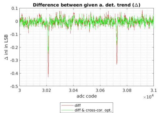
Figure 73 Difference between given and determined INL trend
