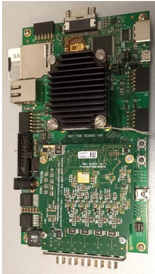
Figure 33 (Superseded) first FC2.0 prototype setup (with “FmcAdc100M14b4cha” as FADC card). The first setup could use the Trenz Modules “TE0720-03-1CF”/ “TE0715-04-30-1C”. The Trenz Module is covered by its black heat sink.
