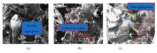
**Figure 11.** SEM images of dry hybrid composites at different graphene weight ratios: (a) Filled with 0.5%; (b) filled with 1% and (c) filled with 1.5%.
