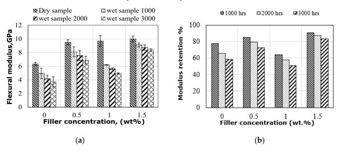
Figure 8. (a) FM under dry and wet environments and (b) FM retention.
