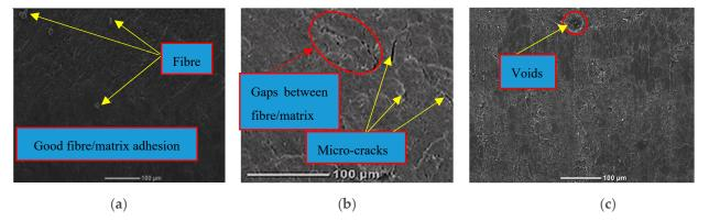
**Figure 12.** SEM images of wet hybrid composites at different graphene weight ratios: (a) Filled with 0.5%; (b) filled with 1% and (c) filled with 1.5%.
