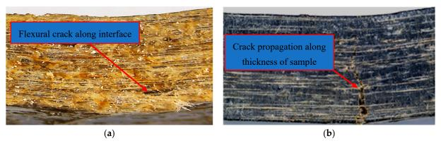
**Figure 7.** Failure of hybrid composites under flexure in wet conditions: (a) Unfilled composites and (b) filled composites.
