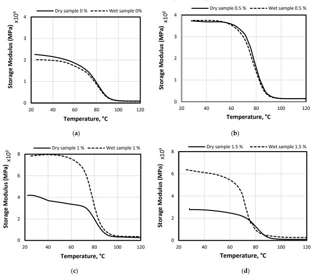
**Figure 4.** Storage modulus of dry and wet samples: (a) Samples with 0%; (b) samples with 0.5%; (c) samples with 1%; (d) samples with 1.5%.
