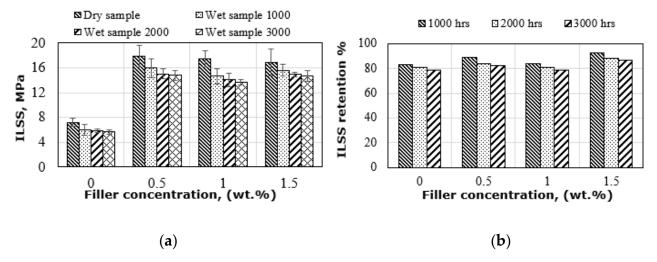
Figure 9. (a) ILSS strength under dry and wet environments and (b) ILSS strength retention.
