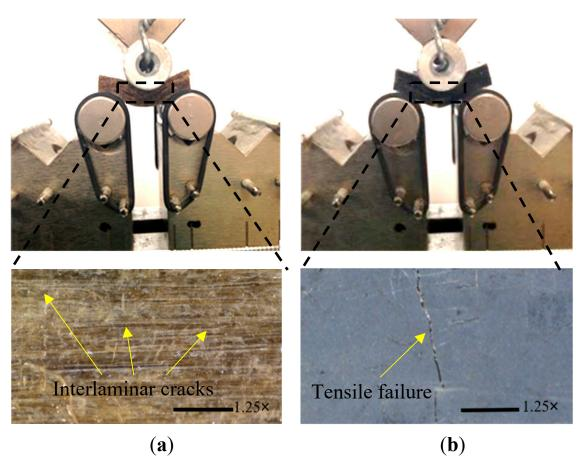
**Figure 10.** ILSS failure of hybrid composites under wet conditions: (a) Composite without graphene and (b) composite with graphene.
