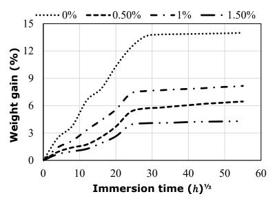
Figure 5. Moisture absorption behaviour of hybrid composites with various graphene weights.
