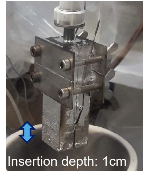
Sample before (left) and after (right) insertion in hot Na bath
