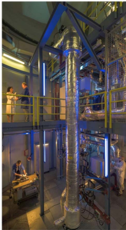
Convection test section Height ~ 6m
