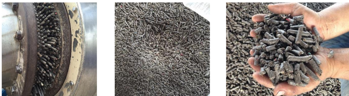
Figure 6. RDF pellets, densified-RDF or RDF-5 (Source of images: Suranaree University of Technology, SUT).
