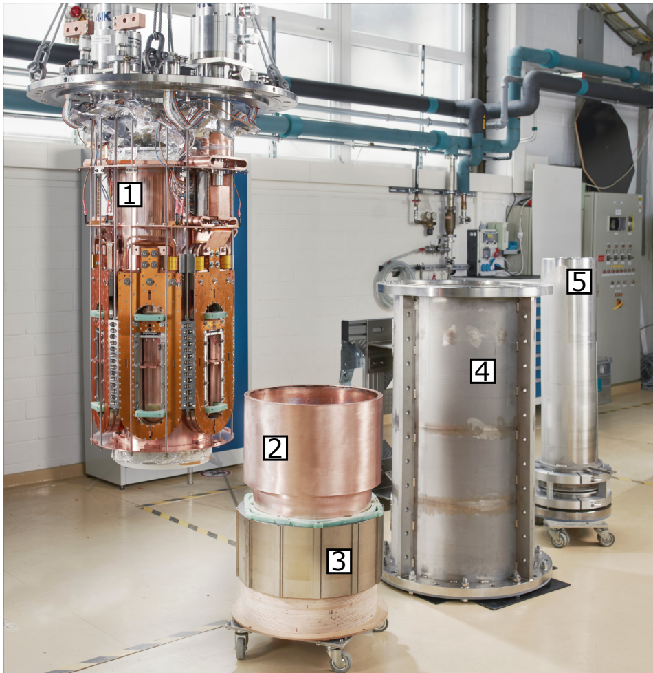
Figure 6.11: Individual components of the generator before assembly. Stator system and inner thermal shield attached to the cryostat top lid [1], outer thermal shield (without MLI) [2], stator iron [3], outer cryostat [4], inner cryostat [5] (Ref.: Amadeus Bramsiepe )
