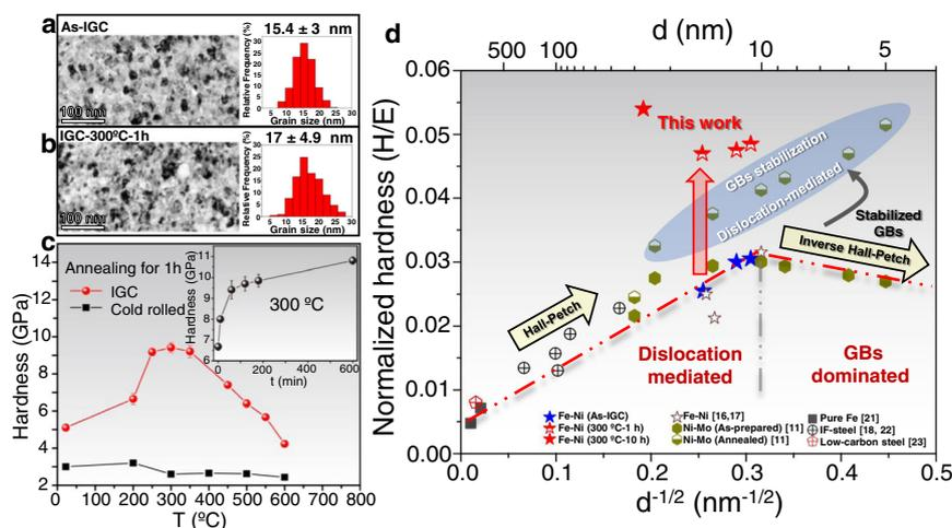
**Fig. 1 | Nanograined Fe-Ni alloy fabricated by IGC and the effect of annealing.** **a, b** Bright-field micrograph and grain size distribution of the IGC samples before and after annealing at 300 °C for 1 h. **c** Microhardness as a function of annealing temperature for the IGC nanograined Fe-Ni and cold-rolled Fe-Ni alloys, and the
