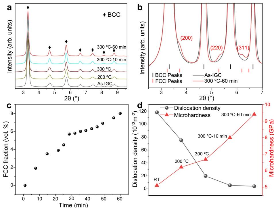
**Fig. 3 | In-situ synchrotron XRD results of the IGC nanograined Fe-Ni samples. a, b** Synchrotron XRD profiles of the IGC Fe-Ni sample. **c** Evolution of the fraction of FCC phase during isothermal heat treatment at 300 °C. **d** Variations of dislocation density and microhardness of the nanograined Fe-Ni sample.
