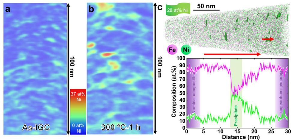
**Fig. 2 | High-resolution chemical analysis of the IGC nanograin Fe-Ni samples.** **a, b** Three-dimensional reconstruction from atom probe analysis of the IGC and annealed (300 °C for 1 h) nanograin Fe-Ni samples. **c** Quantitative linear analysis of the annealed nanograin Fe-Ni sample.
