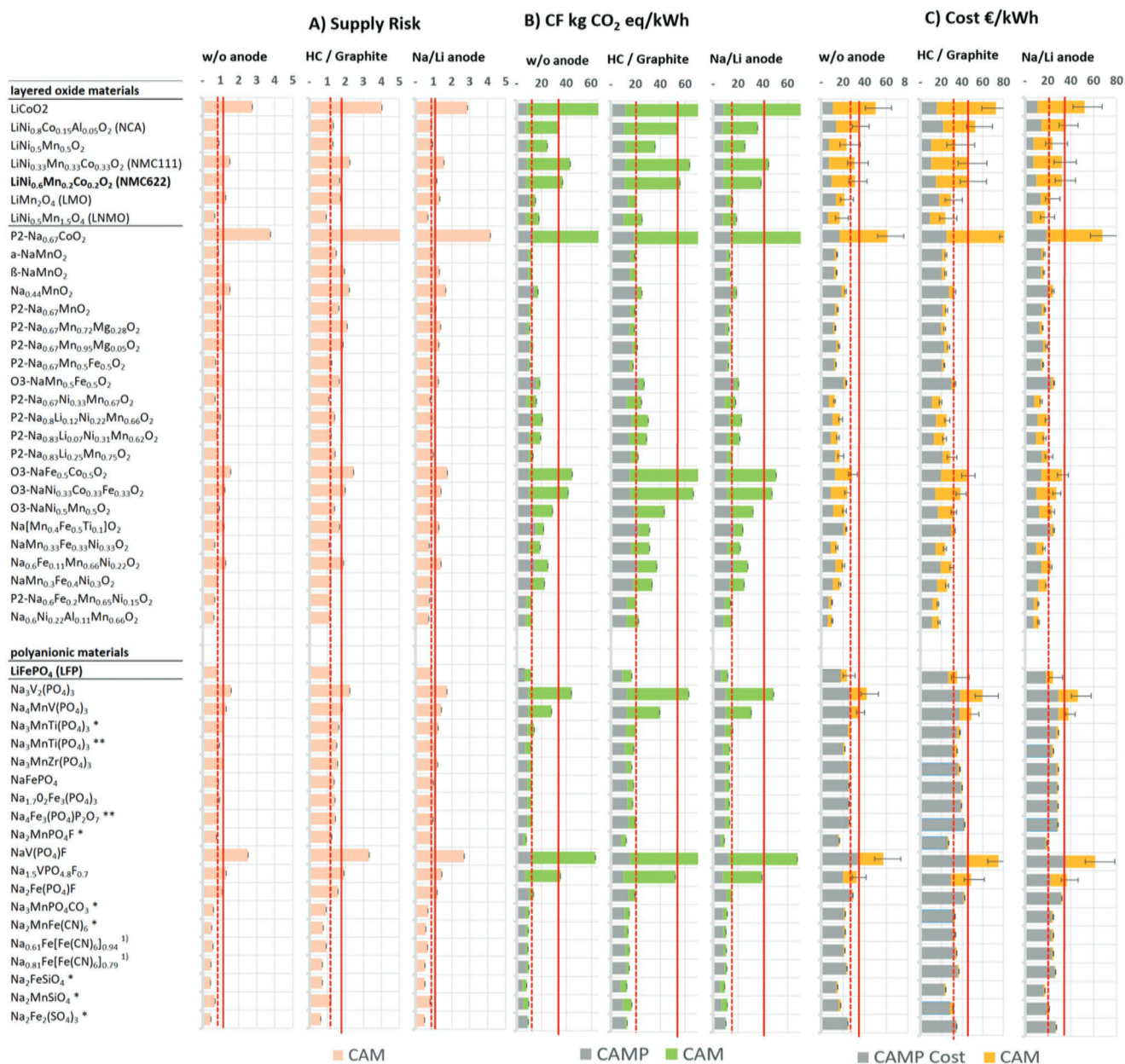
Figure 6. Sensitivity analysis for differing anode materials and changing energy densities for all considered criteria A) SR, B) CF, and C) Cost. Error bars indicate upper and lower boundaries (5 and 95% Percentiles), Indications: a) specific energy is directly from the Literature and the average potential is calculated b) specific energy is calculated from the integration of the potential-capacity, *2Na exchange, **3Na exchange, 1) Prussian Blue Analogues.
