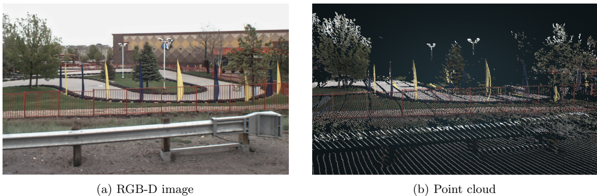
Figure 2.2: Comparison of an RGB-D image and a LiDAR point cloud from the same scene. (Nebiker, 2017)
