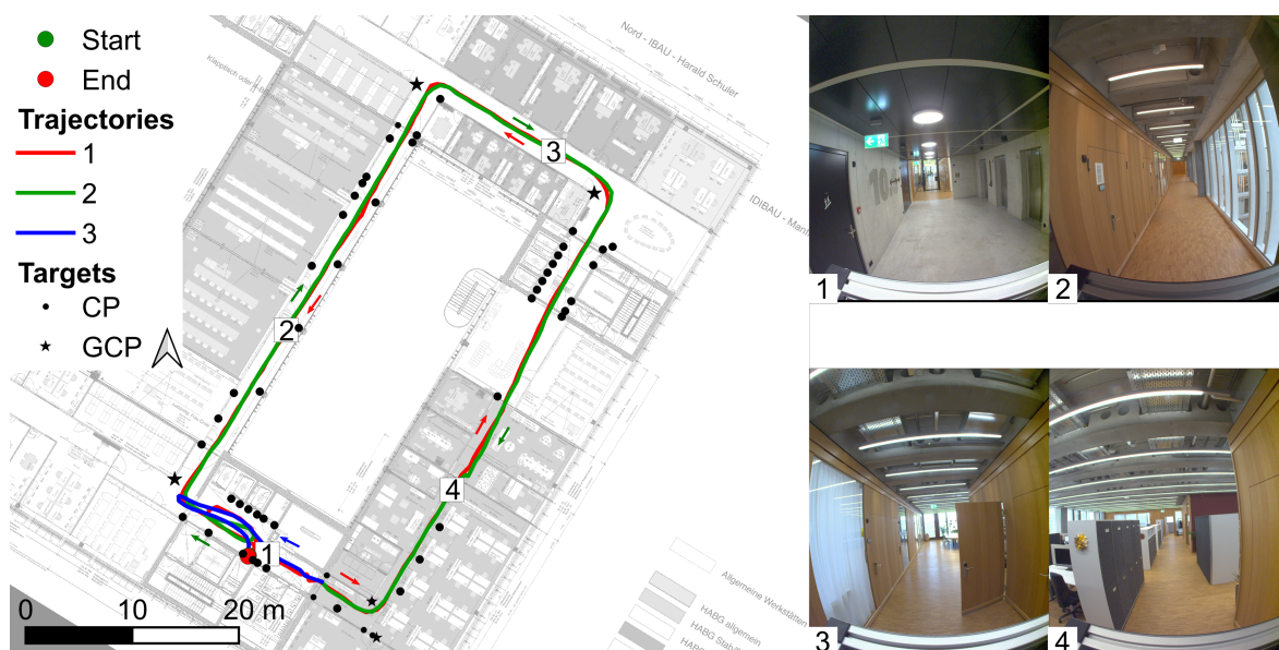
Figure 5.3: Map of the indoor test site located in the FHNW campus nearby Basel with images showing environmental conditions. Arrows in combination with different colored trajectory parts show the moving direction
